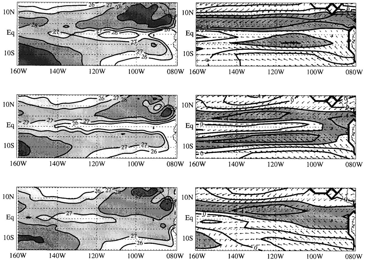
FIG. 6. Time mean (24 Mar–7 Apr) (left) sea surface temperature and (right) surface wind vectors and divergence for (top–bottom) 1995–97. The SST field is contoured every 1°C between 26° and 29°C with values in excess of 26°C shaded. The surface wind divergence field is contoured every  $2 \times 10^{-6} \text{ s}^{-1}$  between  $-4 \times 10^{-6} \text{ s}^{-1}$  and  $4 \times 10^{-6} \text{ s}^{-1}$  with values less than  $-2 \times 10^{-6} \text{ s}^{-1}$  shaded.
