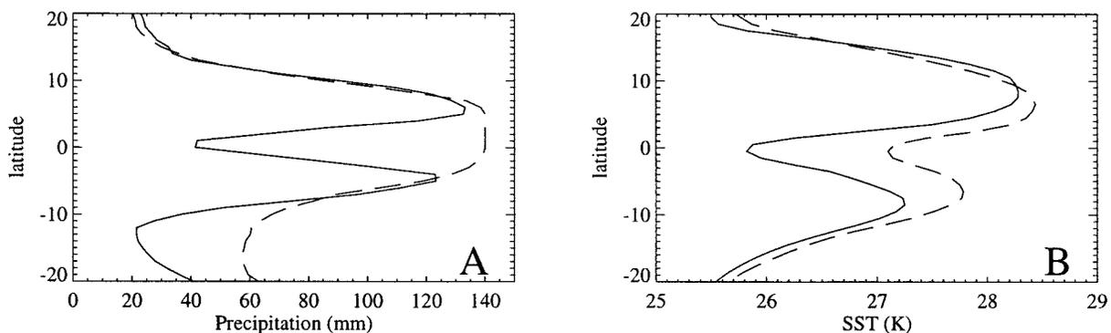
FIG. 3. (a) Composite precipitation and (b) SST for double ITCZ index equal to 1.0 (solid) and for double ITCZ index less than or equal to  $-1.0$  (dash).
